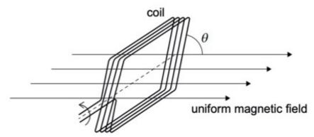
At one instant the plane of the coil is at an angle q to the direction of the field. The magnitude of the emf induced in the coil is
